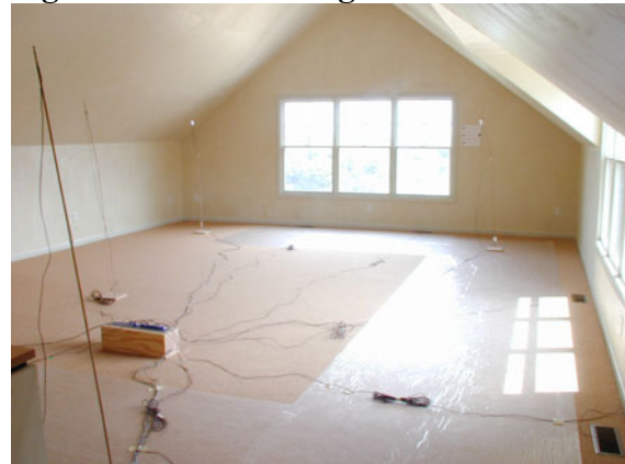
Figure 6. Loft Showing Sensor Placement
