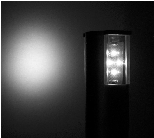
Figure 4. The redesigned LED pole with LED packages mounted behind a thick block of clear acrylic, which is integrated into the aluminium pole. Note that the number of LED packages could be reduced from ten to four due to use of higher-brightness LEDs.
