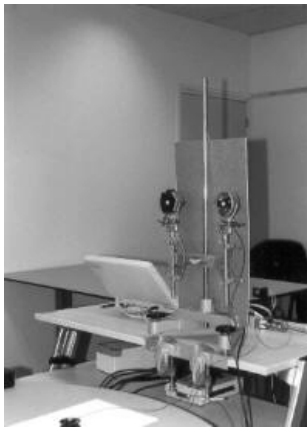
Figure 3: Experimental set-up: facing straight ahead (a) and facing 25° downward (b)
