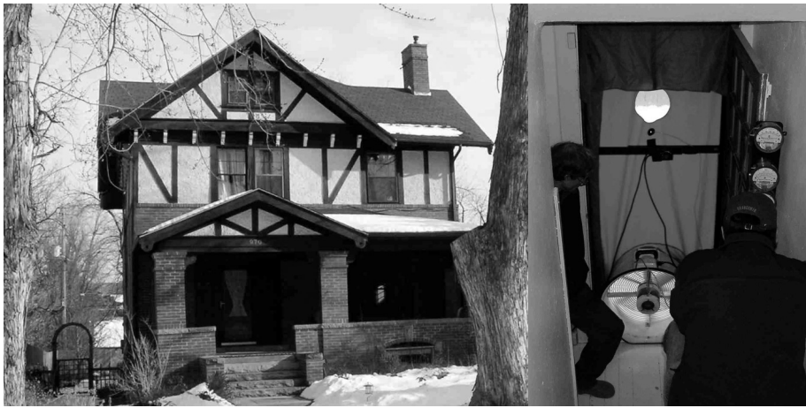
Figure 5. This home is quite leaky as shown by the blower door (right photo), but needs no porch insulation.
