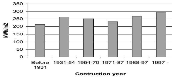
Figure 3. Commercial office buildings and level of annual metered energy use divided into construction year (314 buildings with total floor space 2.4 mill m 2 )
