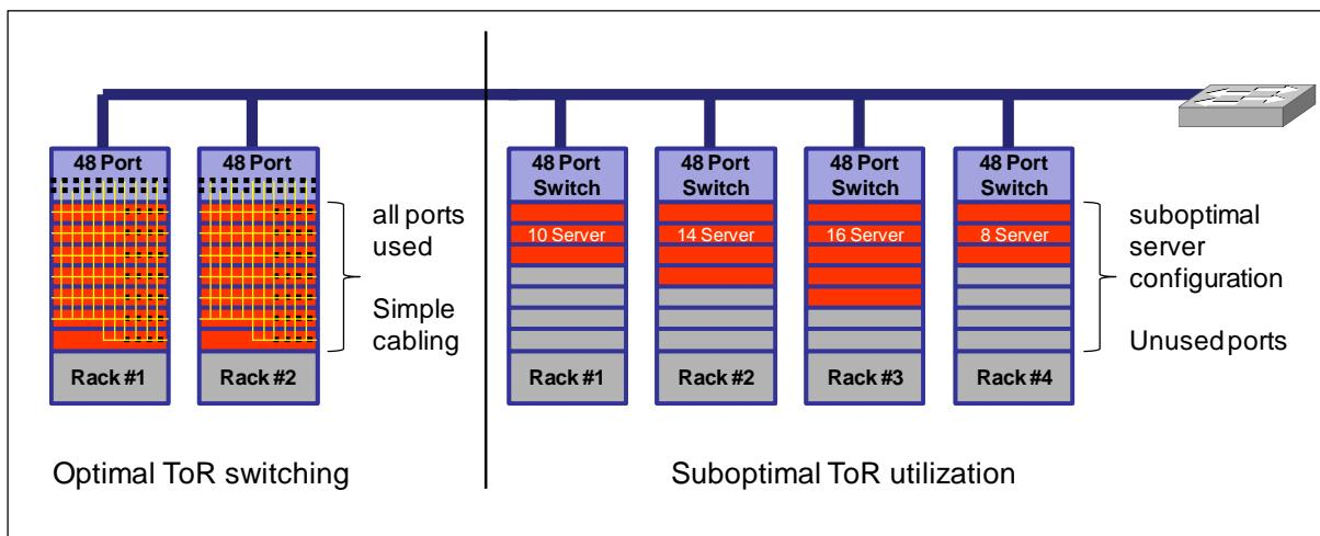
Figure 25: Top-of-Rack switching
