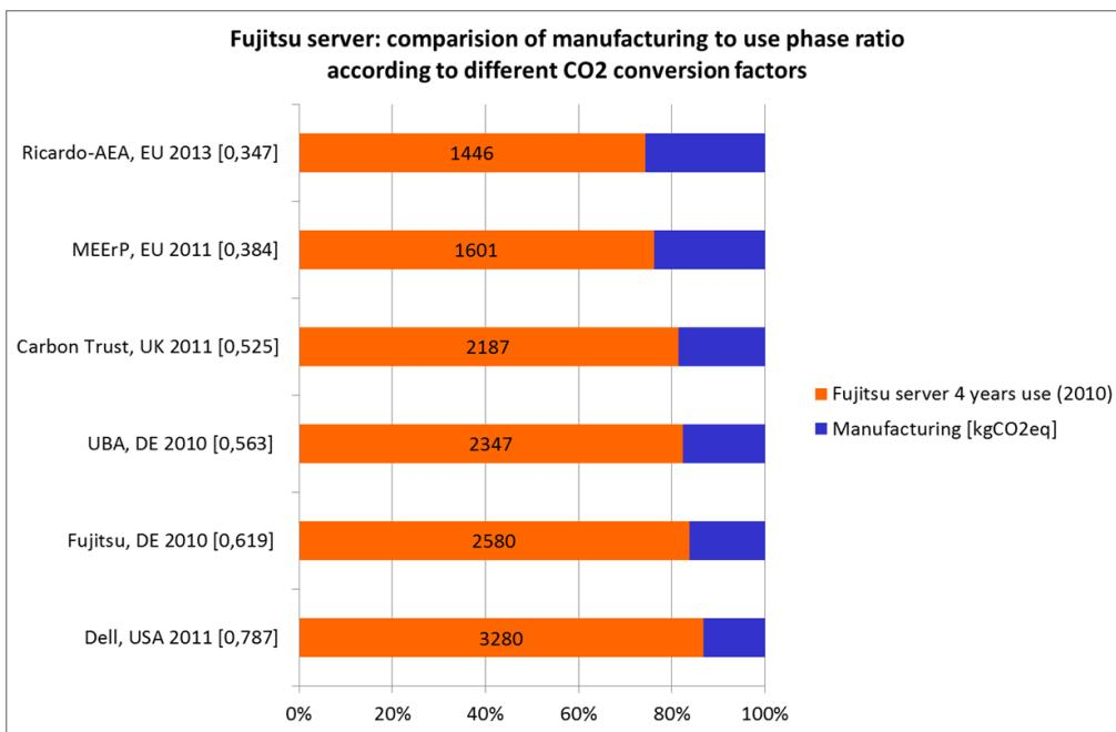
**Figure 2: Calculation of the Fujitsu server PCF with different CO<sub>2</sub> conversion factors**
