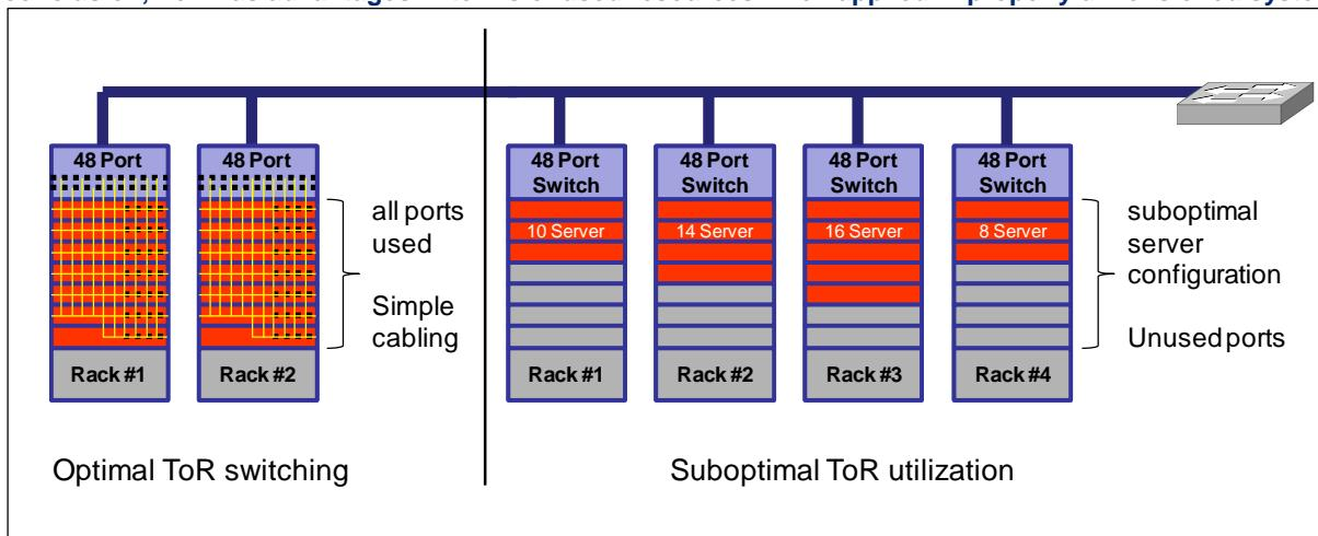
Figure 25 below illustrates the ToR switching concept and its proper utilisation.
