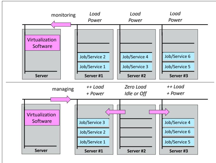
**Figure 21: Schematic diagram of server virtualisation (highly simplified)**
