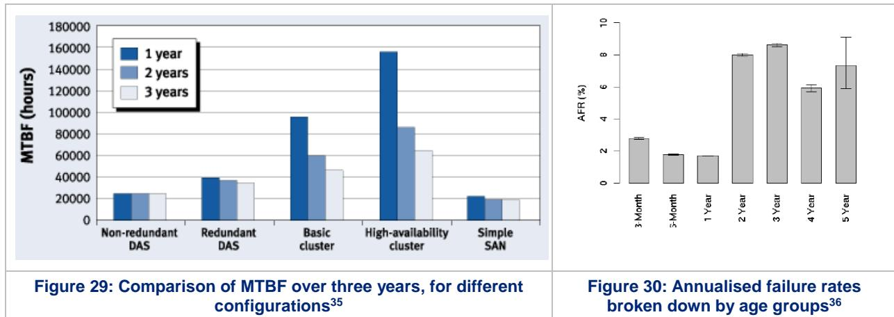
Figure 29: Comparison of MTBF over three years, for different configurations<sup>35</sup>
