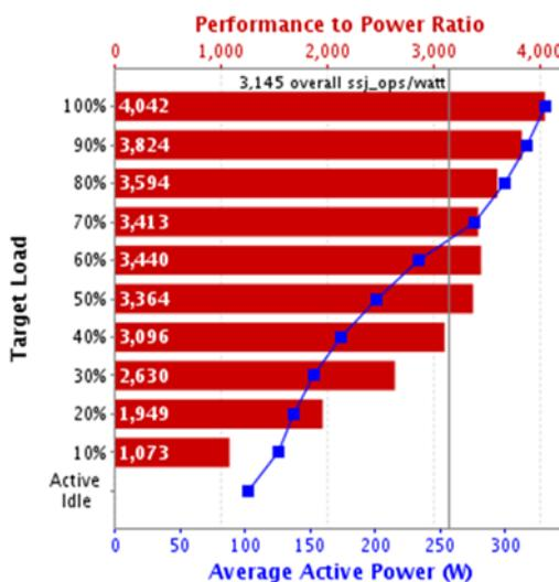
Figure 16: Example of a SPECpower assessment result (2012)
