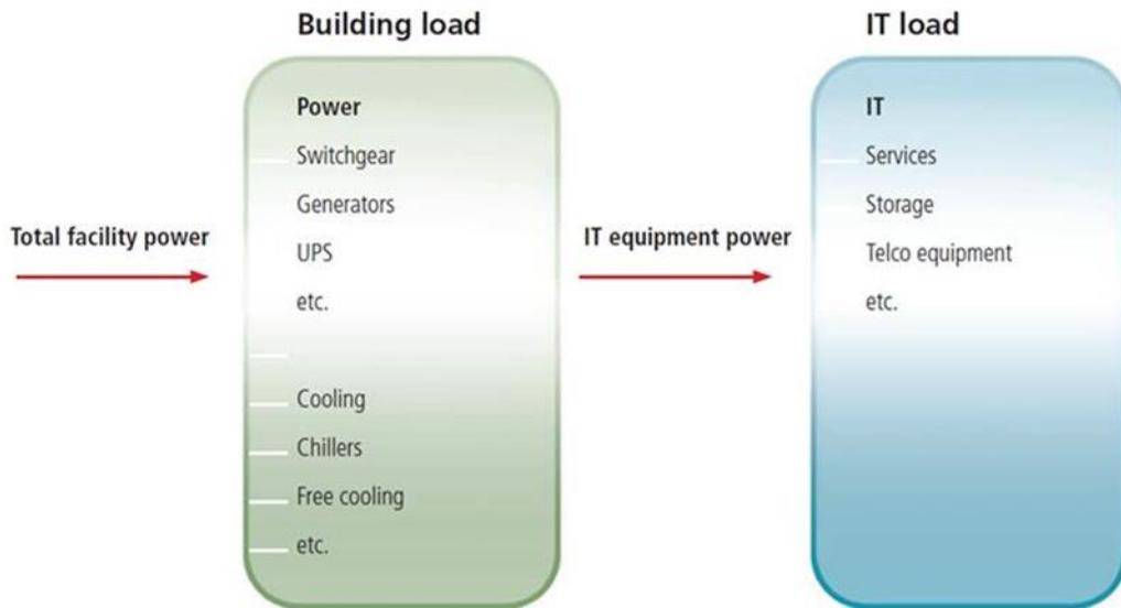
**Figure 26: Typical equipment used in a datacentre, for the calculation of the PUE**
