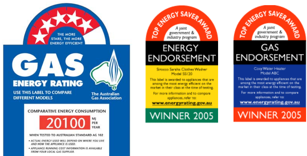
Figure 27-2. Australia mandatory star rating label (left) and TESAW label for electric (mid) and gas appliances (right) [www.energyrating.gov.au]
