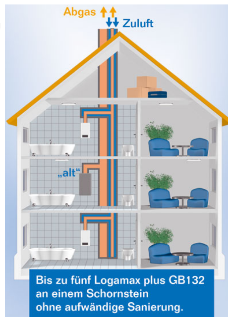
Figure 6-2. Buderus solution for combining old boilers and new condensing ones in a single chimney (with separate flue gas and air shaft).
