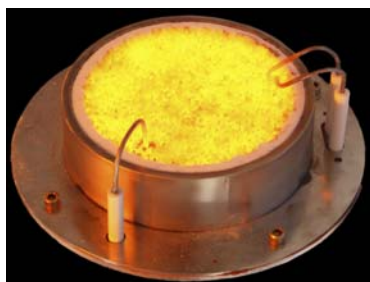
Figure 4-4a. Porous ceramic burner (SiC). Maximum load: 300 W/cm 2 . Modulation range: 1:20. Thickness 15 mm. Low CO: <20 mg/kWh and low NO x : <20 mg/kWh, also during burner cycling operations (on/off). Picture left: www.poreos.com
