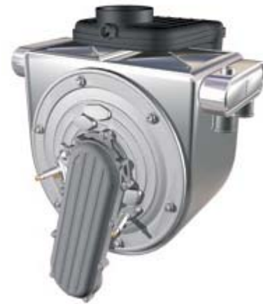
Figure 5-12. The casing (or shell) of the spiral flat tube exchanger. Casing holds the 4 connections for the two media (flue gas and water) and mounting plate for the concentric burner (source: Giannoni).
