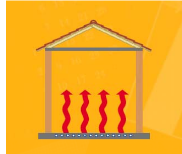
Figure 9-17. Heat distribution with radiation systems
