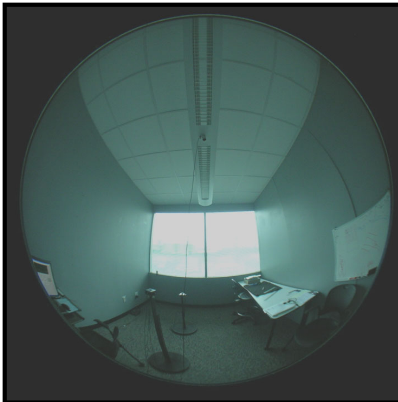
Figure 5. A Fish-Eye View of the Daylighting Laboratory of the California Lighting Technology Center, Showing the Fixture-Mounted Customized Photo Sensor of the SDH Prototype and the Various Photo Sensors Measuring Work Plane and Eye Level Vertical Illuminance Levels
