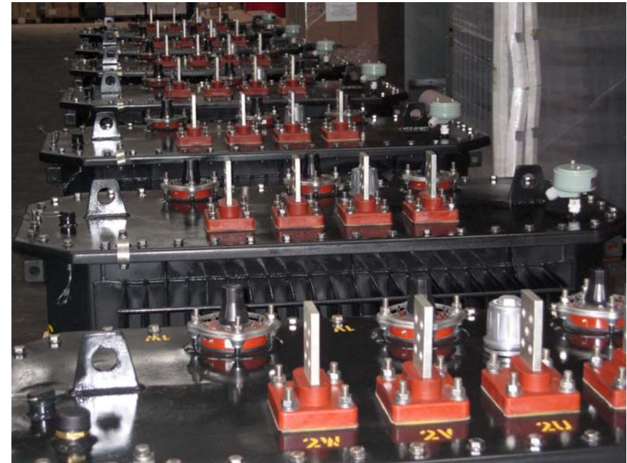
Source: Endesa (Test of 10 amorphous distribution transformers in Mallorca in 2008)
