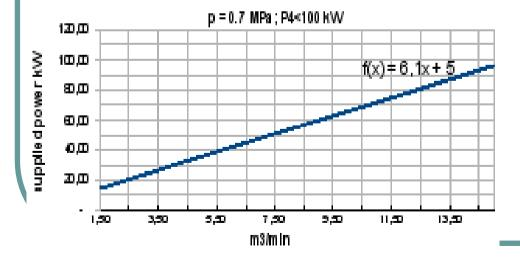
Proposed universal curve, relating capacity and supplied electric power ( $p_{set}$ =0.7 MPa,  $P_4$  < 100 kW)
