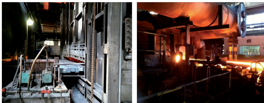
Figure 3. Billet charge inlet and discharge of the reheat furnace.
