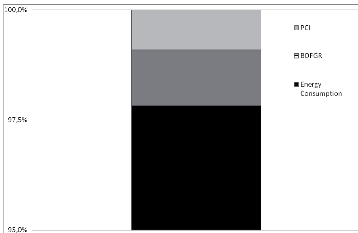
Figure 4. Remaining energy efficiency potential (2012) due to the further diffusion of the selected EET. The specific primary energy per ton crude steel could be reduced by 2.1 % if the selected technologies reached complete diffusion (1.2 % BOFGR, 0.9 % PCI).
