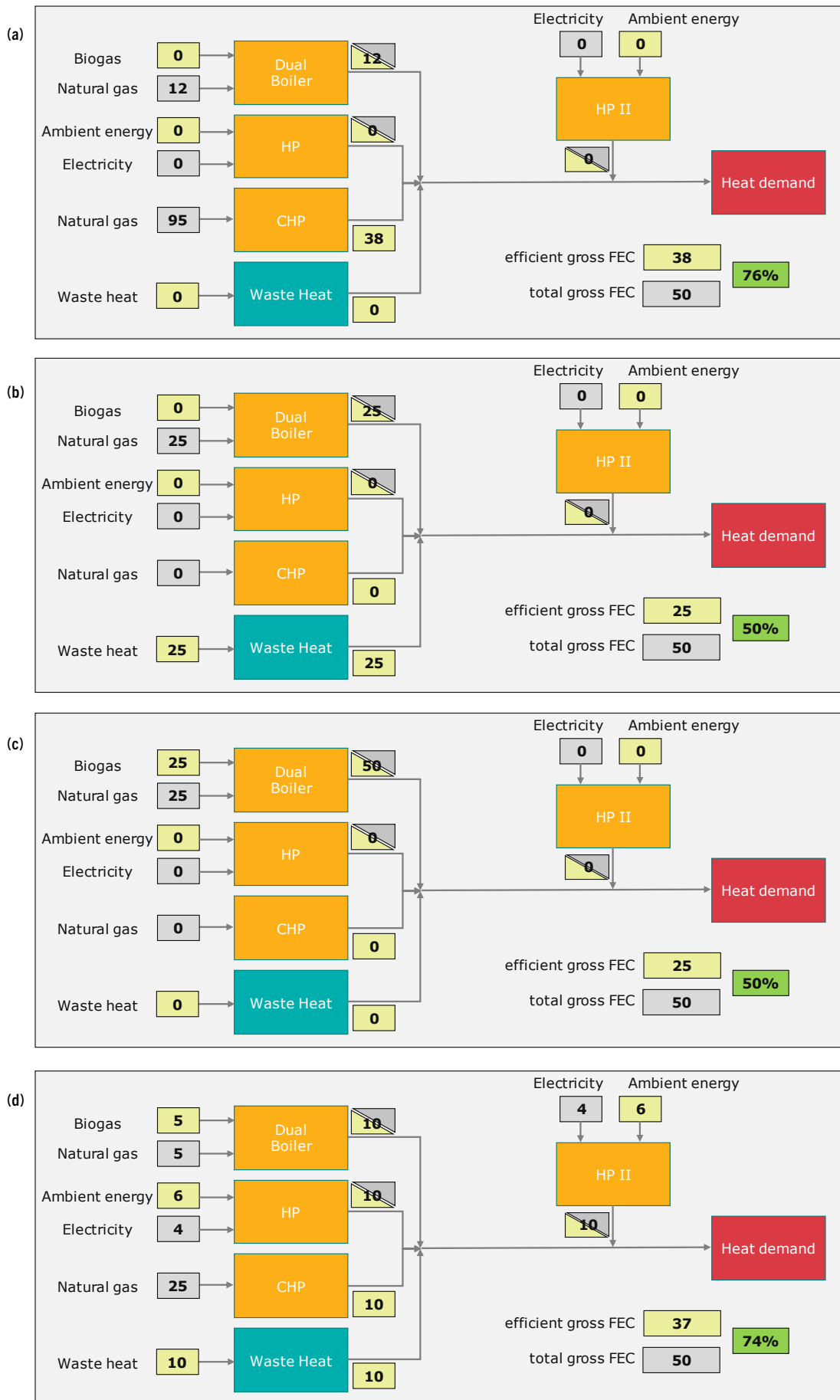
Figure 4. Mock examples of efficient district heating and cooling under the different alternatives (a) 75 % cogeneration, (b) 50 % renewables, (c) 50 % waste heat and (d) 50 % combination.
