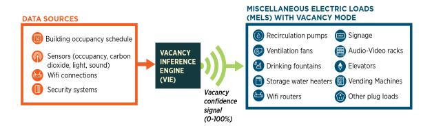
Figure 5. Proposed method to reduce miscellaneous electrical loads in a building.
