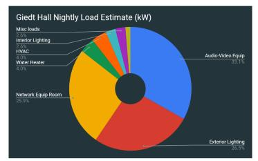
Figure 4. a) Giedt Hall electricity use and Wi-Fi connections; b) Estimated electricity end-use breakdown in Giedt Hall during vacant periods.
