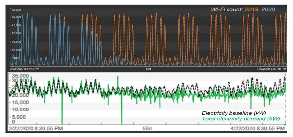
Figure 2. UC Davis electricity consumption before and during the pandemic, with counts of Wi-Fi connections shown to demonstrate drops in occupancy.
