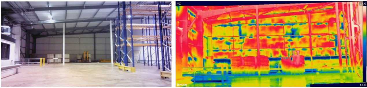
Figure 1. A mid-construction building, early in the build process, in photo and thermal image. The blue areas (cold, according to the temperature scale to the right of the thermal image) show where insulation has slumped within the wall, after installation. This is a defect that can be seen clearly only in the thermal image which has been thermally tuned.
