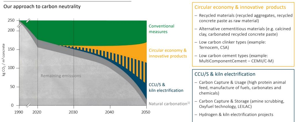
1) Natural carbonation is the absorption of CO<sub>2</sub> from the atmosphere during the lifetime of a concrete construction
