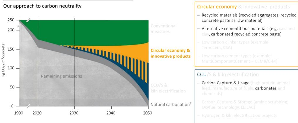
1) Natural carbonation is the absorption of  $CO_2$  from the atmosphere during the lifetime of a concrete construction
