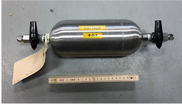
Figure 4. WP1-3. Left: Water heater D on a test bench. Bottles with calibrated gases ( CO , NO , NO_2 ) are sent to laboratories for a blind test (laboratories do not know the composition).
