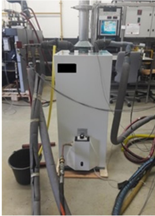
Figure 4. WP1-3. Left: Water heater D on a test bench. Bottles with calibrated gases ( CO , NO , NO_2 ) are sent to laboratories for a blind test (laboratories do not know the composition).
