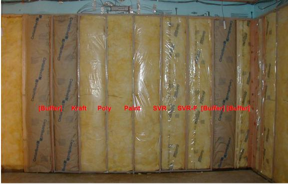
Figure 3. Test Walls, South Orientation, Pre-Drywall (West Walls Similar)
