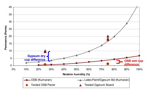
The test results at wet cup conditions for painted gypsum board are similar to published data. However, at dry cup conditions—closer to the wintertime operating conditions—the tested permeance is much higher, averaging 9.8 perms (compared to 3.1 perms in the literature). Although the tested specimen would meet requirements for a Class III vapor retarder, it was much higher than expected.
