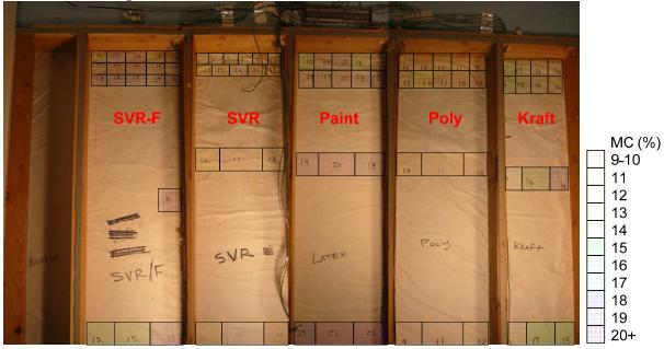
Figure 8. Moisture Content Distribution in West Test Walls
