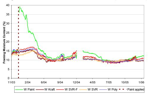
Figure 7. Sill Plate Moisture Content for West Walls (Outboard Side)
