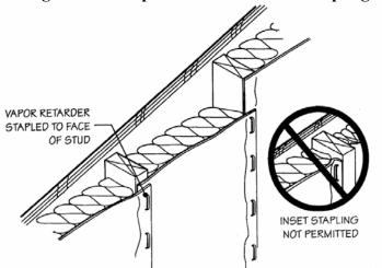
Figure 1. Examples of Face and Inset Stapling
