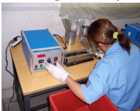
Liquid Mercury Dosing Technique Source: Banwell 2005
