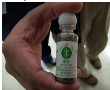
Mercury Pellets (Solid Dosing Technique) Source: Banwell 2007
