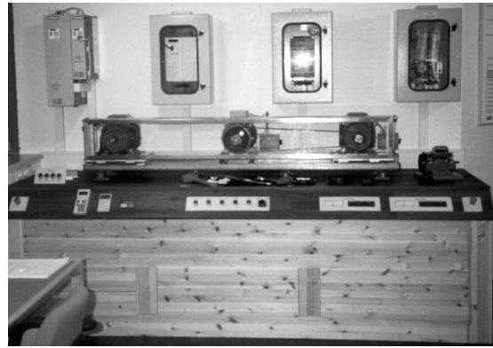
Figure 3: The Optimization of Belt-Driven Motor Systems campaign test facility built by TRE-FOR.
