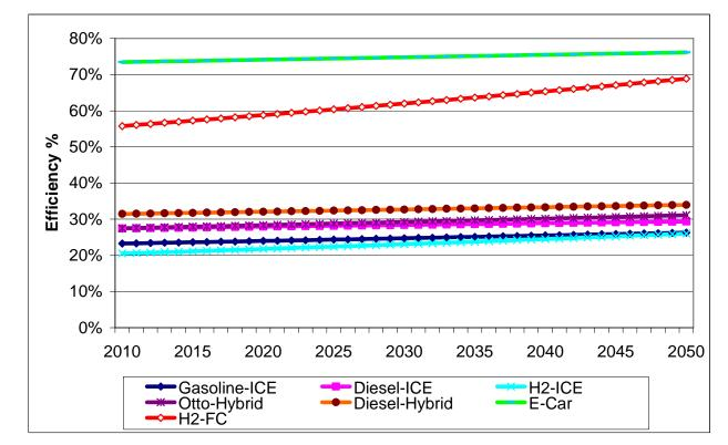
Assumptions on the development of efficiency of the analysed vehicles 2010-2050 (Source: AVL)
