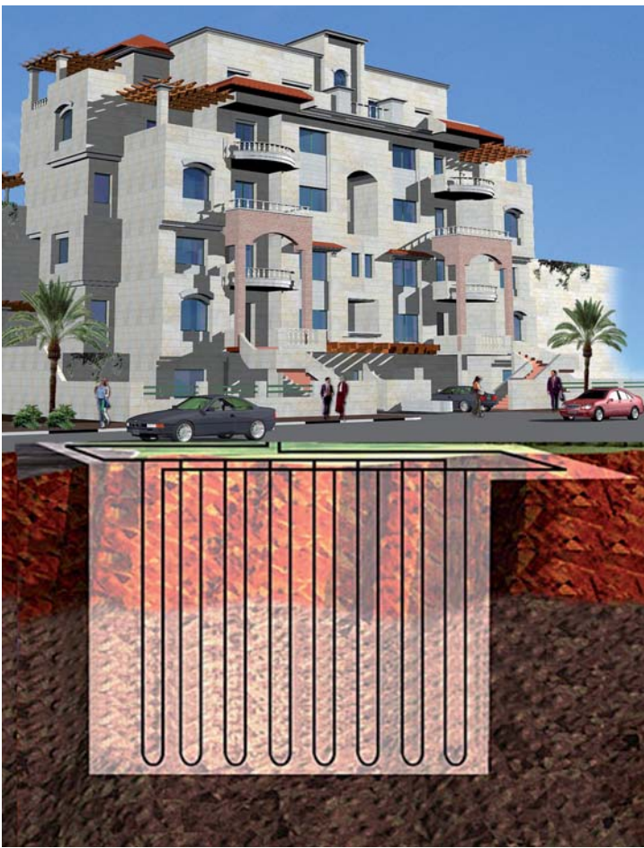
Figure 2. Vertical Ground Heat Exchanger at Model Villa
